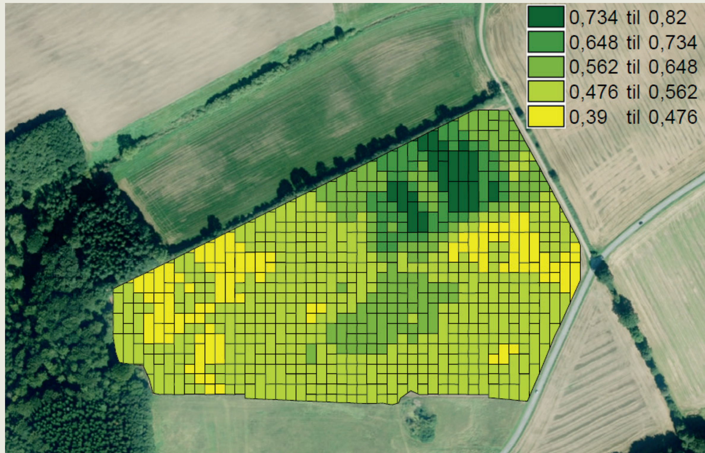
FIGURE 1. An example of an NDVI map with 10x10 m cell grid in a field growing catch crops.
